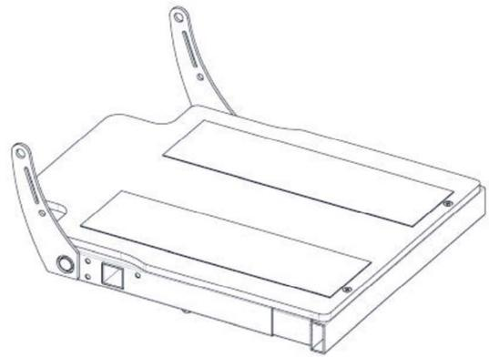
The Flex-II seat is fixed directly to the base frame.
