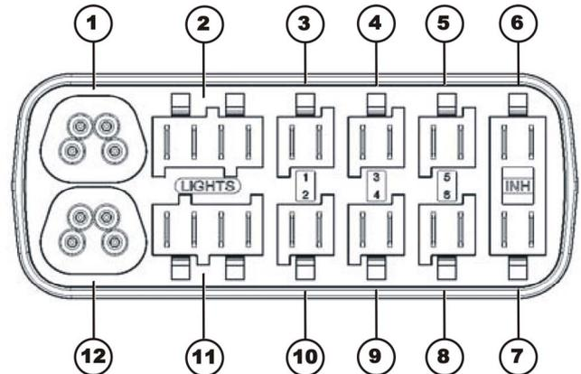
\* The INH connection is used for actuator limitation or speed reduction.
