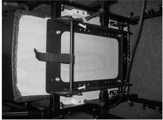
The fixed seat is fixed directly to the base frame.
