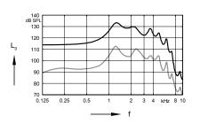
Output sound pressure level (L<sub>i</sub> = 90 dB)
