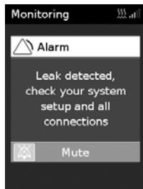
When an alarm is activated, the yellow LED alarm indicator will flash, the alarm will sound and a message will appear on the screen.
