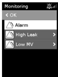
If multiple alarms are activated at the same time, the most recent alarm message will be displayed on the screen and any other activated alarms will be shown in the Alarms list.
