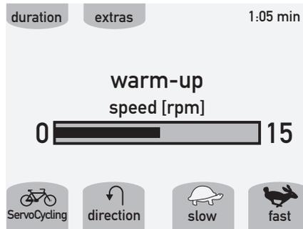
The speed automatically increases (Pre-setting: leg trainer warms up to 15 rpm, arm/upper body trainer warms up to 5 rpm). Without pressing any further buttons the motor of the MOTomed gracile12 will gently move your legs in a safe way.
