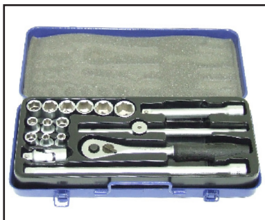
Reversible ratchet and socket wrench inserts size. 8-24
